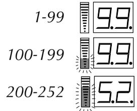
4. If you are using a T-Max® 1A or 3A as a "master" remote, the "id" of the sunbed must be set to "1". If you are using a T-Max® Manager each sunbed must be assigned a different "id". To set the "id" press the timer button, to count up, or the body fan control button, to count down, until the desired number is achieved.
