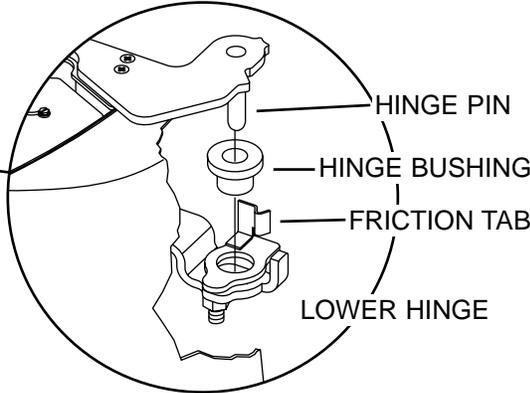
Place the Hinge Bushings into the hinge holes (top and bottom). Carefully lower the door hinge pins into the bushings, being careful not to bend the friction tabs.
