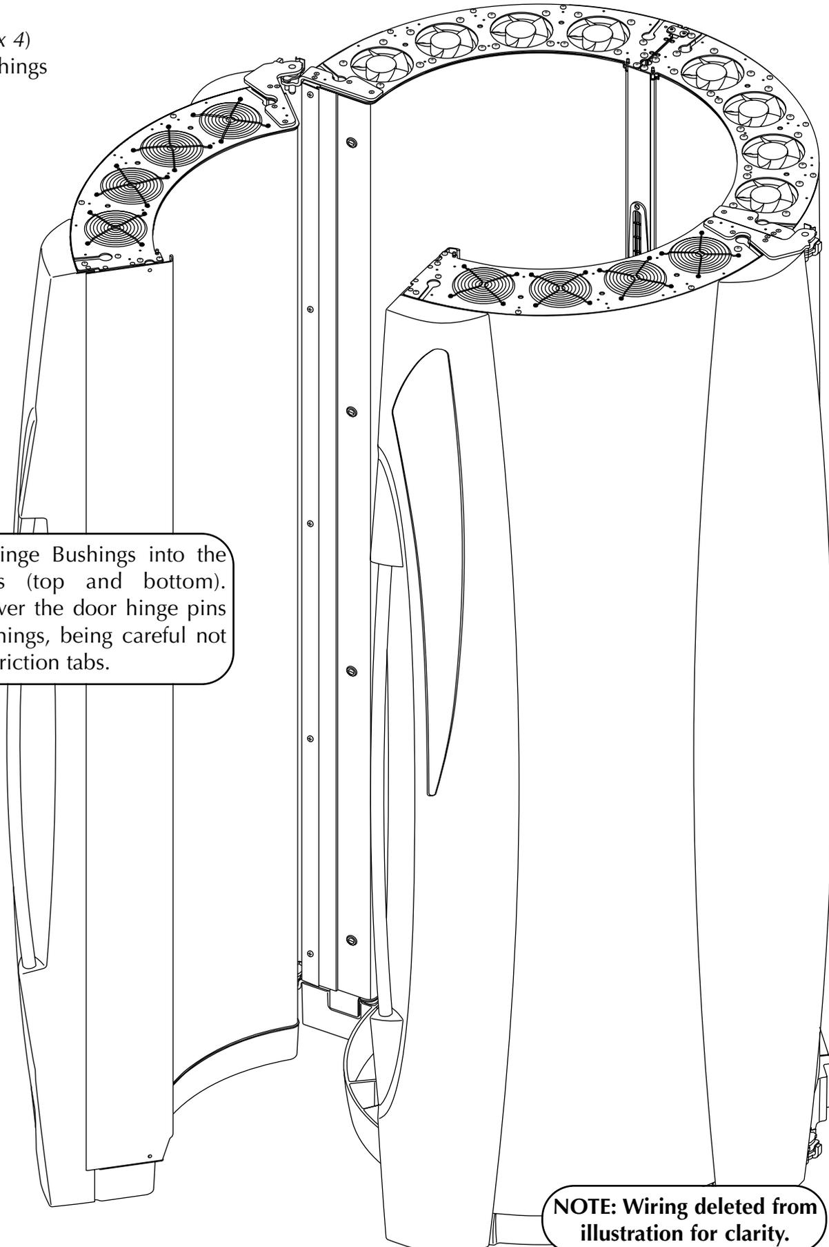
Place the Hinge Bushings into the hinge holes (top and bottom). Carefully lower the door hinge pins into the bushings, being careful not to bend the friction tabs.
