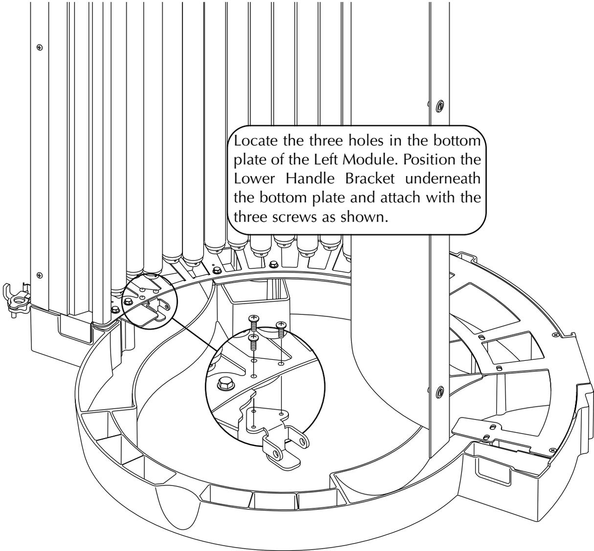
Locate the three holes in the bottom plate of the Left Module. Position the Lower Handle Bracket underneath the bottom plate and attach with the three screws as shown.
