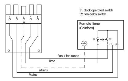
A 2 or 3-minute "Lag Relay" after-cooling timer should be connected in all commercially employed solaria. This function is standard on most remote timing devices developed for use in the indoor tanning industry, or can be ordered from your authorized distributor as an easy-to-install module.
