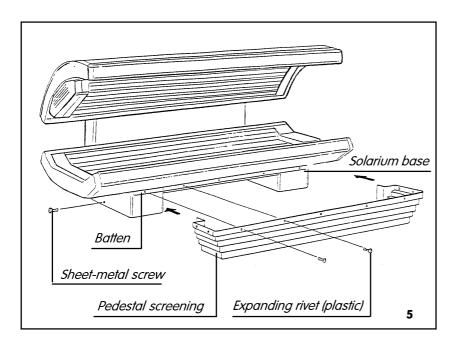
The actual pedestal screening is not fitted until the unit has been fully assembled, with bed and canopy fitted.
