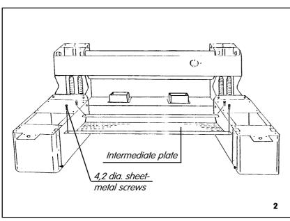
Then attach the intermediate plate supplied, as illustrated in Fig. 2, to the solarium bases, using four of the 4.2 dia. x 9.5 sheet-metal screws supplied.
