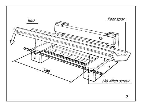
The bed must now be lifted by two persons, lamp side uppermost, so that the spar with the openings points to the rear. Guide the tabs projecting from the openings into the rectangular openings in the column bases and then lay the bed - while still pressing it gently towards the rear - on the bases.
