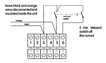
A 2 or 3-minute "Lag Relay" after-cooling timer must be connected in all commercially employed solaria. This function is standard on most remote timing devices developed for use in the indoor tanning industry, or can be ordered from your authorized distributor as an easy-to-install module that fits onto the main contactor block, and is connected to pole no. 6 (red) there on.
