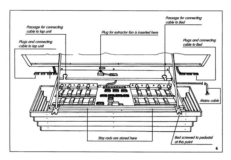
Lastly, connect the mains cable to the power supply by mean of a CEE plug and socket, or by permanent connection. Lower the bed onto the pedestal again, after removing the stay rods, which can be stored in the front recess of the pedestal. Once the bed has been screwed to the pedestal with the M6 screws supplied, the sunbed is ready for operation.
