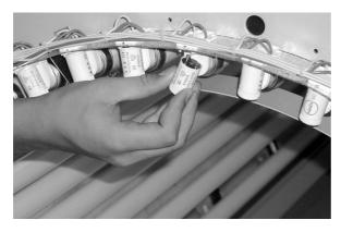
For easier replacement of the starter remove the side screen.
