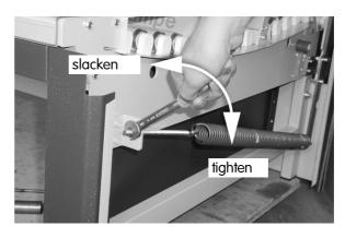
Turning right means to tighten the spring stronger, turning left means slacken the spring.
