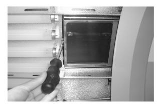
Now the filter box is folded out and removed slanted to the center of the equipment.
