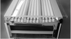
Now the fixing metal for the acrylic sheet will be put at the back side of the bench on the acrylic sheet and will be screwed with the back socket covers. To guarantee that you can pull the acrylic sheet out of the cam in the fixing metal, lie below each cam a mountage angle with PE-protection foam cut as vertical setting.
