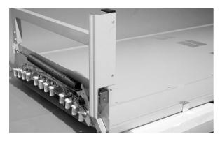
Between the foot elements the back socket cover will be screwed. Please pay attention that the rounden edger at the cover is at the same level with the longitudinal girders at the bench.
