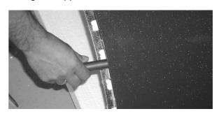
With these transport movements you can now hang in the canopy at the back fixtures of the bench. At the same time you have to lift a little bit the canopy at the front.
