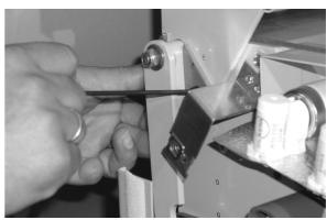
Now mount the side covers of the canopy with the necessary special screws on the right and left assembly outside.
