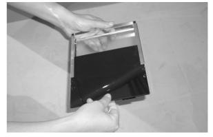
Please note that the filter inserts must always be installed at the correct position to the metal halogen lamp. The blue filter disk must face the side where the metal halogen lamp is located.
