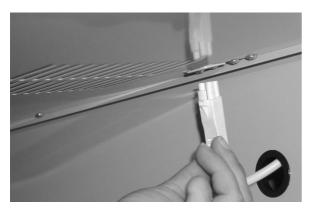
Finally the assembly with the connecting lead will be connected with the power supply network.
