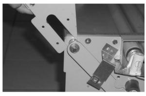
When the canopy is hang in, the safety strap has to be mounted at the left and right canopy suspension. Set the respective safety strap from the below side in the suspension and screw it on 3 positions per side at the canopy.
