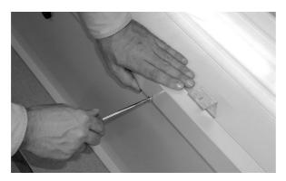
The 4 enclosed angles for fixing the stand covers now have to be screwed on both outsides of the side covers of the bench. In this case the nut has to be placed always on the upper position of the angles.
