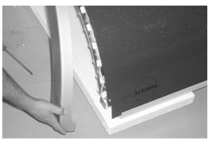
Turn now the attached assembly help in the planned thread at the behind place in the head brace at the left and right canopy side.
