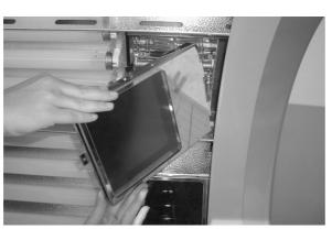
For cleaning and replacement of the filter inserts remove the locking plates at the support tracks. Now you can remove the filter inserts without problems.
