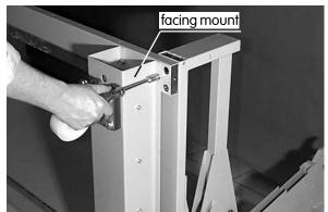
3. Disconnect the front and back longitudinal beam from the stands. Do this by removing all 8 screws (hex head M12, SW 10) from the corners.
