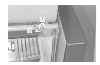
The lamp frame can now be swung onto the acrylic bench plate. Lamps and starters are removed or replaced from or into their sockets by turning them 90 degrees.
