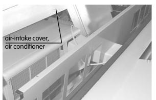
3. In addition, the metal cover panel over the controls in the middle pedestal area must be unscrewed.
