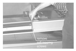
2. Afterwards, remove the inside metal casing covering the two cooling fans for the lamp area. Do this by releasing all screws from the front as well as the lower areas of the air-intake shafts.
