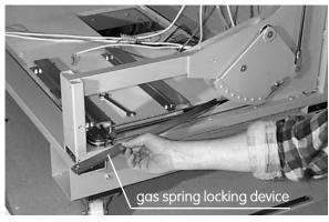
Pull the canopy down until the gas spring locking devices can be hung into the screws on the front curved segments. Insert the cable binder into the latch to keep it from coming open again.
