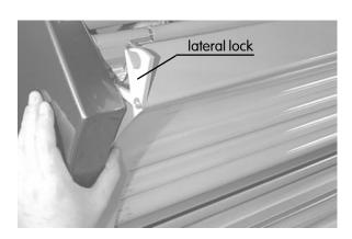
Now swing the pane frame forward and pull it upwards to remove it at the pivot points.
