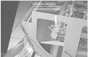
4. Please note that 3 cooling fans are attached to the facing. Because of this, you must first release the fan connection cables at the attachment clips before lifting the facing out of the unit. The safety clips can be released with a screwdriver.
