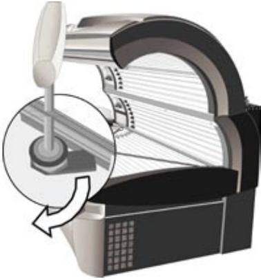
The sunbed acrylic rests in a profile groove in the front and rear side and across its whole length. Two sash locks secure the sunbed acrylic against unauthorized removal. The sash locks are opened with the help of an Allen key (6mm). A safety switch controls the installation and position of the sunbed acrylic.
