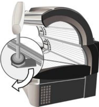
At the front and rear side, across its whole length, the sunbed acrylic sits in a profile groove. Two sash locks secure the acrylic against unauthorized opening. The sash locks are turned by an Allan key (6 mm). A safety switch controls the installation and position of the sunbed acrylic.
