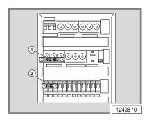
In case of circuit breakers which cannot be unscrewed, a strip of adhesive tape may be applied over the actuation lever (1 + 2) with the wording 'Do not switch, danger!'.
