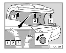
Remove the 2 lamps above and the 2 lamps below the interior lighting.
