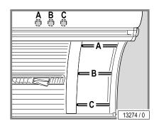
The facial tanner's UV low pressure lamps must be removed first so that the UV high pressure lamps and the filter panels can be changed.
