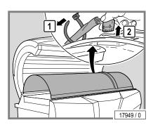
The canopy panel must be completely removed from the device in order to replace the lower, long UV low pressure lamps.
