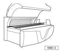
Open the panel and lay it down carefully.
