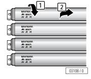
UV low pressure lamps possess a reflector which directs the light outwards. The lamps must be mounted in such a way that the rear side of the reflector is located on the device side.
