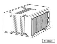
Use a fin comb to clean the air conditioning's dirty cooling fins.
