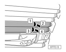
Remove the 2 lamps above the interior lights.
