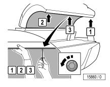
Remove the screws and then remove the lamp cover.
