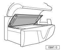
Remove the lamp covers at the head and foot ends.
