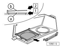
Fit the new filter panels in the correct sequence.
