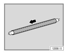
Slide the sleeve onto the new lamp.
