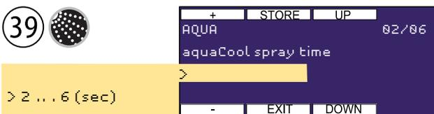
Determines the duration of the aquaCool spraying time.
