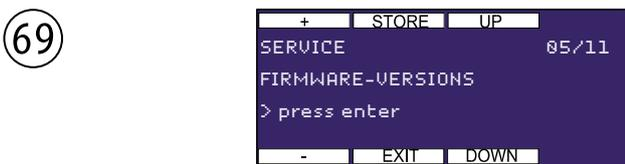
Submenu call with START/ENTER. Displays the current firmware version of the system components.
