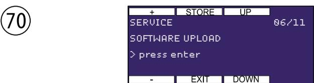
Submenu call with START/ENTER. Displays the first and the last Software-Upload.
