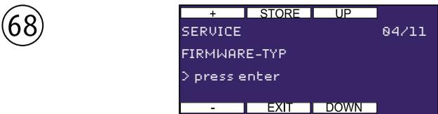
Submenu call with START/ENTER. Displays the current firmware typ / variant.
