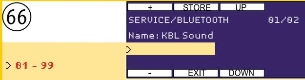
To fit your Studio environment (multiple units) different numbers can be added to the bluetooth device name (KBL Sound **xx**) of each solarium.
