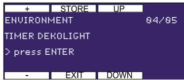
Entering switching times for the decorative lighting. The submenu is invoked by pressing START (ENTER).
