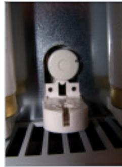
Installing the tubes: Make sure that the inscription on the tubes is visible, for otherwise, there will be no tanning effect.
