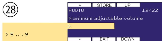
Presetting the maximum adjustable sound level, limits the maximum adjustable sound level in the operating and standby mode.
