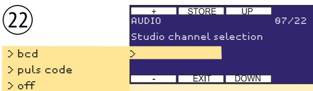
Allows for the change-over between pulse-code and BCD-code mode with the Studio signal pending and deactivates the external-channel selection.
