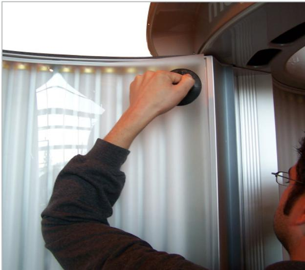
Take hold of the pane from behind and release the right-hand side in a downward movement. The pane can then be removed.
