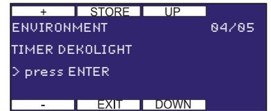
Entering switching times for the decorative lighting. The submenu is invoked by pressing START (ENTER).
