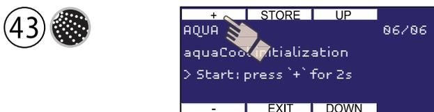
Starts the aquaCool initialization process. A spraying cycle of 90 seconds is started to bleed the system before commissioning, after a repair operation or after a canister replacement.
