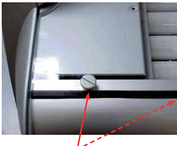
Fig. 3-4 Undo the two screws of the base pane
