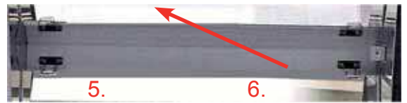
Abb. 3-8 Clamping springs retaining the filter panes
