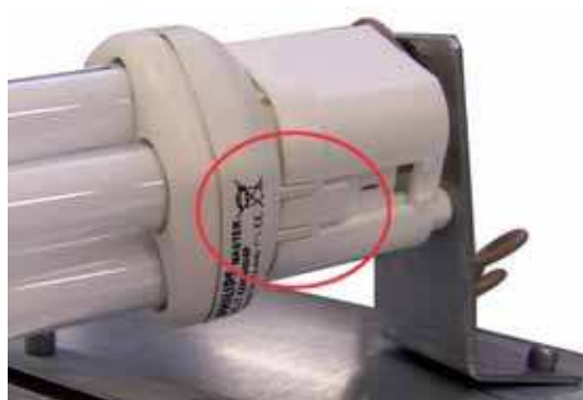
Fig. 3-6-7 Correct position of the connector
