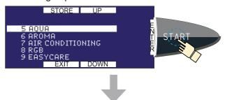
The currently active function (circle) is displayed in the centre line on the left-hand side. You can invoke further functions of this group by pressing 4 (UP) or 9 (DOWN).
