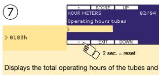
includes a reset function and set function to set the value in steps of five via the +/- buttons.
