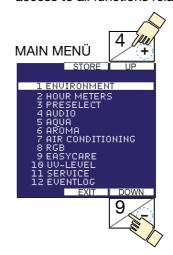
• Select the desired function group from the main menu by pressing the 4 (UP) or the 9 (DOWN) button. The currently selected group is highlighted.
