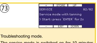
The service mode is switched on for 10 minutes. The mains voltage is connected. Error notifications are ignored, tanning can be started. After this period, there is a 3 minute restart lockout.
