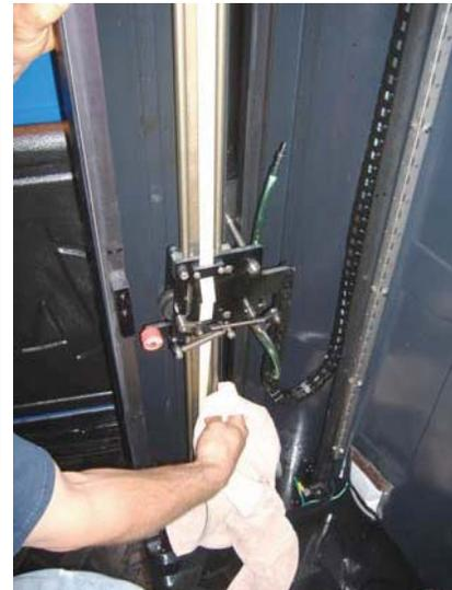
Before purging the nozzle, use rubbing alcohol or glass cleaner and a rag to clean the rider rail. Make sure you clean the front and back side of the entire rail. Pour alcohol in upper sliders and wipe down the rail again. Purge the nozzle by pressing the purge button on the touchpad. After purging, clean the lower section of the rail. Replace back cover, and ring pin to operate unit.
