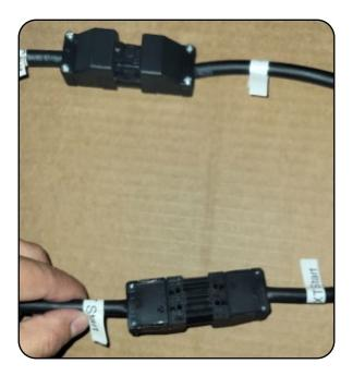
5.4. Unscrew the male connectors coming from the unit and connect the wires coming from the wall using a small flat head Screw driver.
