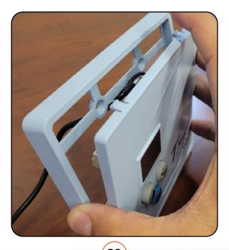
2.3. Using the screws coming with the T-max attach the plastic enclosure
