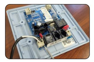
2.2. Separate the T-max Face plate from the internal frame.
