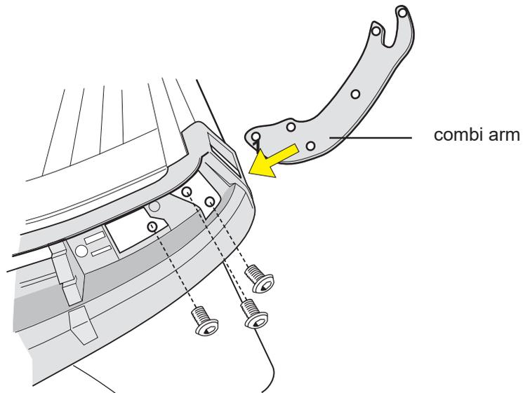
Insert combi arm into bench and secure with screws. Repeat these steps on other side.
