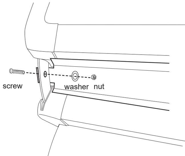
Secure by attaching the *deco shield* to combi arm.
