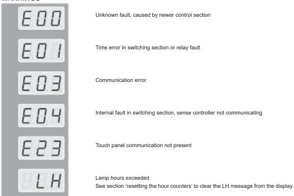
**Note:** When one of the above-mentioned fault messages appears on the display, you should no longer use the device and the unit should be disconnected from the power. Contact ProSun for further instrictions. (This does not apply to the LH message.)
