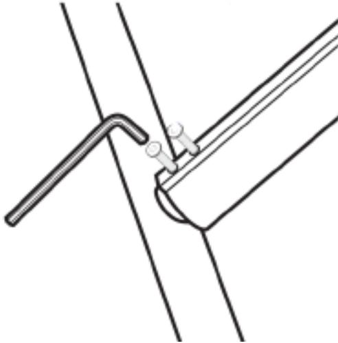
Secure base with allen wrench and two screws
