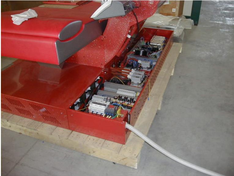
**Rear Equipment Tray Lamp Contactors etc**
