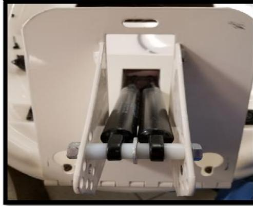
**Figure 7.6.3 Pin Bolt Position on Hinge Assembly.**
