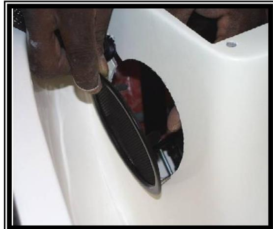
Figure 7.3.3 Removing Heater Intake Screens
