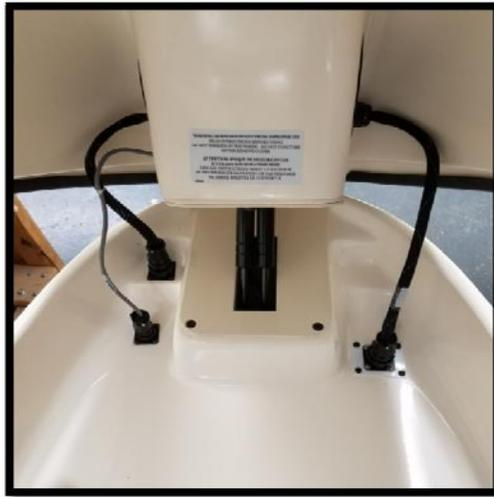
Figure 7.1.1 Releasing Electrical Connectors.
