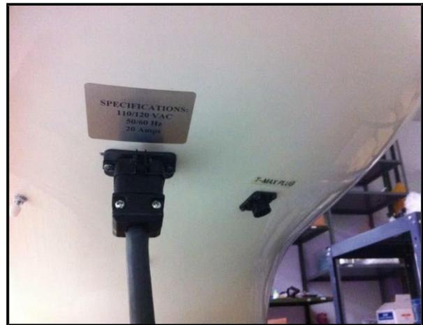
**Figure 4.7.1 Connection of Power Cord.**
