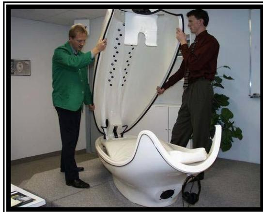
**Figure 7.1.3 Removing the Hood.**
