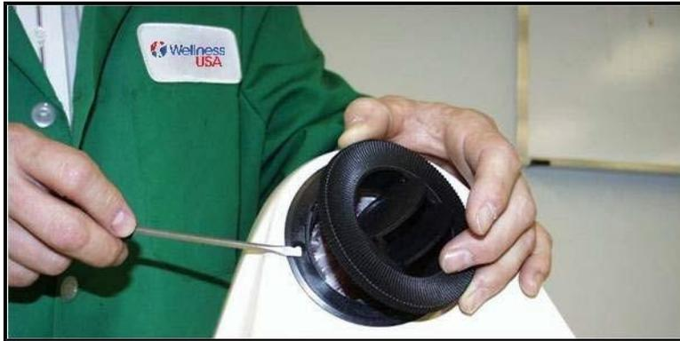
Figure 7.16.1 Removing Face Air Vent(s).
