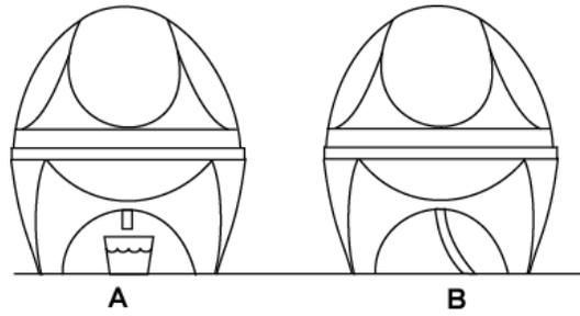
Figures A and B are possible variants to drain the capsule. You can use a water pan to collect water from condensation or connect capsule drainage.
