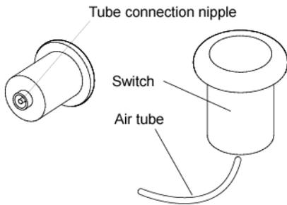
The on-off switch breaks electric input when you press it. A temperature increase could cause the unit to automatically shut off. To resolve this problem, remove the right side skirt and disconnect the air tube from the tube connection nipple on the switch.
