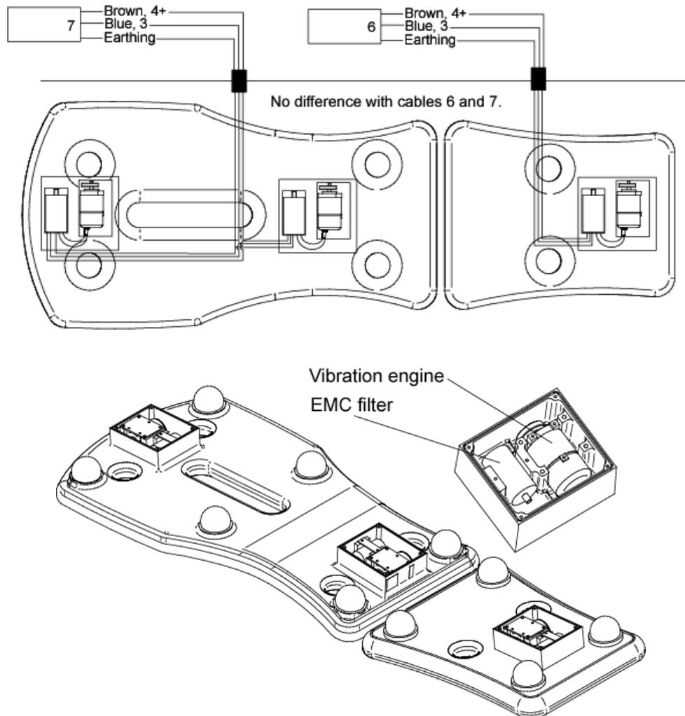
The vibration system has three (3) electrical motors with EMC filters. The motors with filters are connected to special nests on the back of the beds. Two (2) motors and filters are located on the upper bed, and one (1) motor and filter is located on the lower bed.
