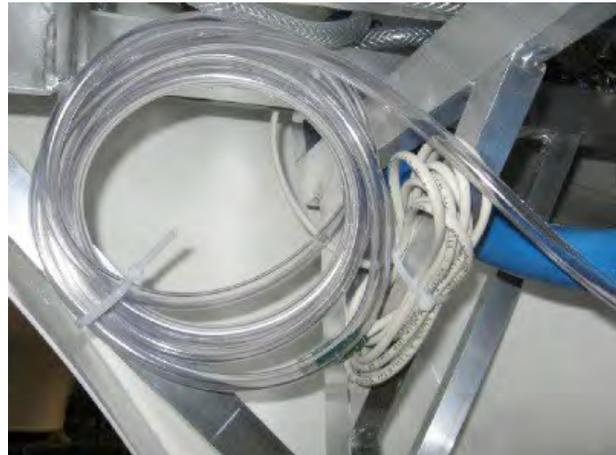
4. Release the tube from the frame by removing the plastic strip. Locate the end of the O<sub>2</sub>-IN tube and connect it with the Oxygen System.
