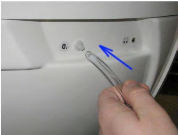
6. O<sub>2</sub> will flow into the capsule through the O<sub>2</sub> nozzle on the hood in the foot area as shown in the picture below.
