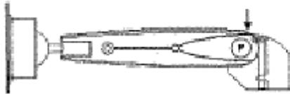
Rising: Adjust the screw moving the wrench clockwise till you reach the desired position. If the unit moves down, adjust the crew moving the wrench counter-clockwise till you reach the desired position.
