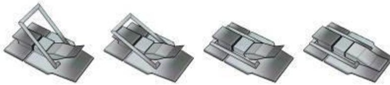
Figure 4.2.3: Latch Locking System
