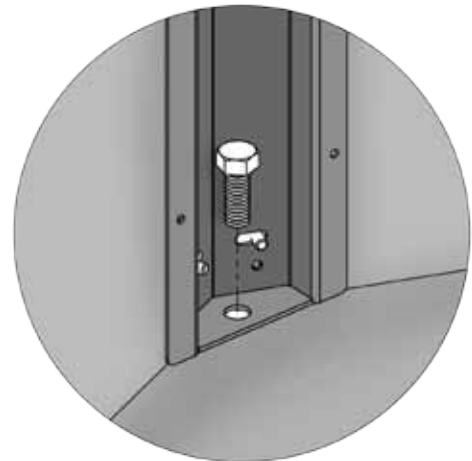
3/8"-16 bolt detail on posts
