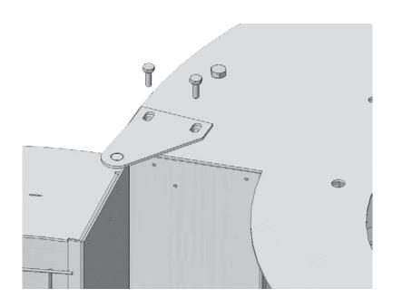
To install door, slide bottom corner of door onto hinge pin located on base of unit. Once door is resting on hinge pin, stand door vertical. Install hinge bracket into top of door section and on studs of top plate. Secure hinge bracket to top plate by tightening 1/4" locking nuts into studs that pass through the hinge bracket.
