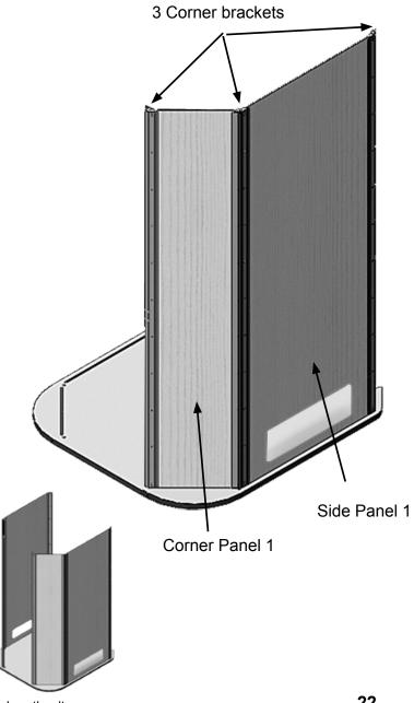
With one person holding the side panel in place, the second person attaches the corner bracket on each side of panel with a 9/16" wrench. Next, attach the corner panel and a corner bracket.
