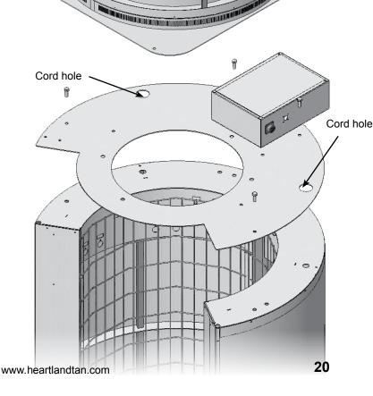
While feeding cords from sections 1 & 2 through cord holes in top plate, place plate on top of sections 1 & 2. Secure by tightening 3/8" X 1" hex bolts.
