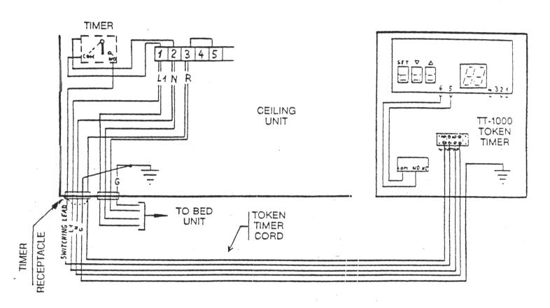
Remove the shorting plug installed in the timer receptacle and connect the timer cord.
